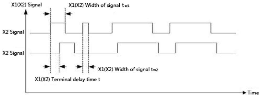
Figure 6-14 X1/X2 terminals delay
